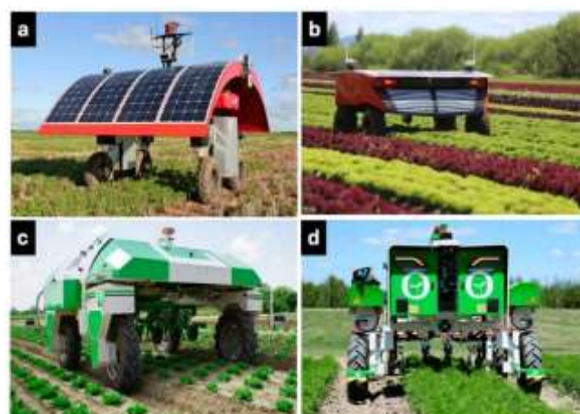
Fig: Spraying robots (a) LadyBird (b) RIPPA; Mechanical weeding robots (c) Dino (d) ORIO.
