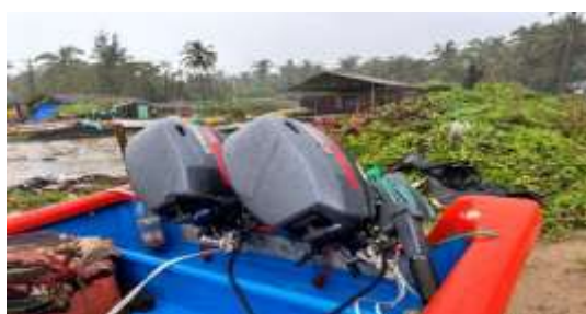
Fig 1. Double engine installed for gill net fishing
