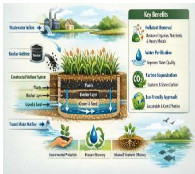
Figure1. Biochar-Integrated Constructed Wetlands for wastewater treatment
