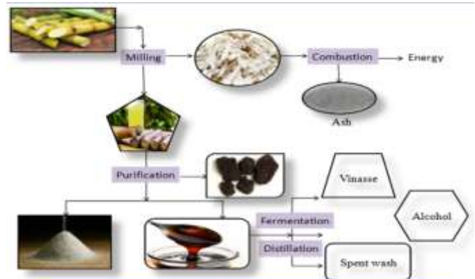
Fig.02: Flowchart of sugar and ethanol production process along with byproducts
